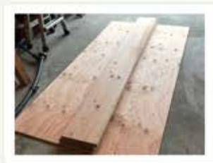
together. (I used 3 inch wood screws. When assembling, its important to work on a flat surface, otherwise your platform won't sit flat on floor under machines.)
